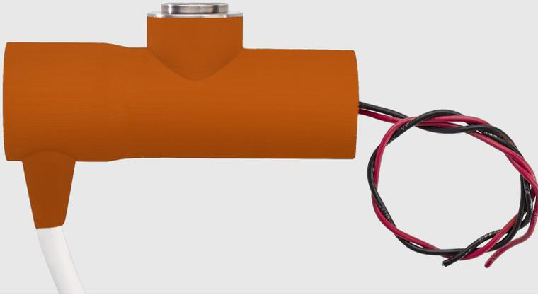
Our Silicon Encapsulated X-ray tube is widely used for thickness gauging applications. This tube includes an electron gun specifically designed to operate for many years at low kV, and high mA. The LGH3 cable is ready to plug into your power supply. Silicon encapsulation provides high voltage isolation as well as a surface to mount your heat sink.
